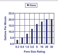
This chart represents typical water flow @ 1 PSID per 10" cartridge length. The test fluid is water at ambient temperature. Extrapolation for multiple elements tends to be linear, but as flows increase the DP of the housing becomes more apparent.
