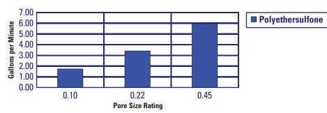
This chart represents typical water flow @ 1 PSID per 10" cartridge length. The test fluid is water at ambient temperature. Extrapolation for multiple elements tends to be linear, but as flows increase the  $\Delta P$  of the housing becomes more apparent.
