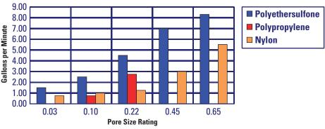
This chart represents typical water flow @ 1 PSID per 10" cartridge length. The test fluid is water at ambient temperature. Extrapolation for multiple elements tends to be linear, but as flows increase the  $\Delta P$  of the housing becomes more apparent.
