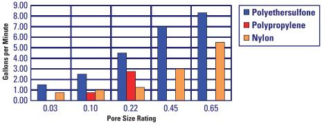
This chart represents typical water flow @ 1 PSID per 10" cartridge length. The test fluid is water at ambient temperature. Extrapolation for multiple elements tends to be linear, but as flows increase the  $\Delta P$  of the housing becomes more apparent. **†Deduct 15% of the flow rate when using a pre-layer of poly depth media**.
